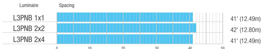
Average spacing for 1 out of every 4 luminaires, normally ON in the path of egress, when at 8, 10, or 12 foot mounting heights.
