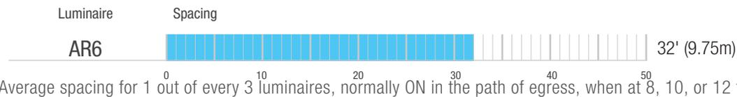
Average spacing for 1 out of every 3 luminaires, normally ON in the path of egress, when at 8, 10, or 12 foot mounting heights.
