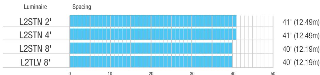
Average spacing for 1 out of every 4 luminaires, normally ON in the path of egress, when at 8, 10, or 12 foot mounting heights.
