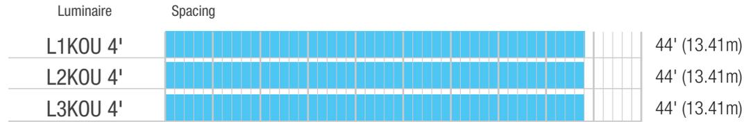
Average spacing for 1 out of every 4 luminaires, normally ON in the path of egress, when at 8, 10, or 12 foot mounting heights.
